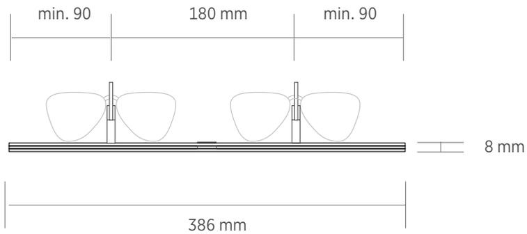
The incredibly thin UniLock shelf (8 mm), made of white acrylic, features a patented magnetic code locking mechanism.
