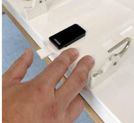
Place the magnetic key on the magnetic field. You have now activated the magnetic-coded locking mechanism.
